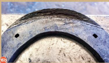
15. Once you have a shape that is nice and elliptical, line up your bar and toe on the anvil and use it as a square to draw a clean line at the back edge of the web. Take your time and mark your nails when the shoe is cold (this is the most important part). Place a nail hole behind the back edge of the toe bend, at the widest part of the shoe, and split the difference. The nails will ideally exit center of stock.
