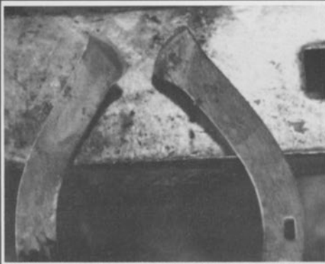
8. Properly scarfed, swelled out, and thin on ends. Again, keep scarves short.
