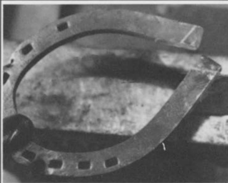
3. Use an anvil devil or hardy to mark both heels.
