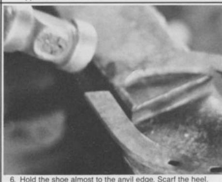
6. Hold the shoe almost to the anvil edge. Scarf the heel. Note thumb position on the side of handle. For a good weld, keep scarf short.
