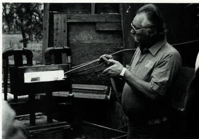
Miller makes welding aluminum in the firepot look easy.
