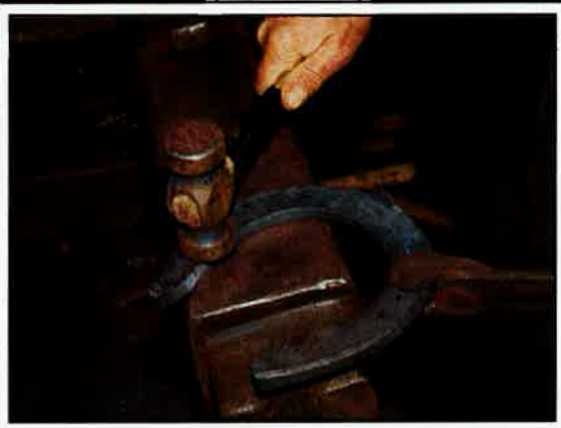
After back punching and before leveling, the round end of the hammer should be run around the inside edge of the foot surface to make sure it does not impinge on the sole when fit. This applies to most shoes with few exceptions.
