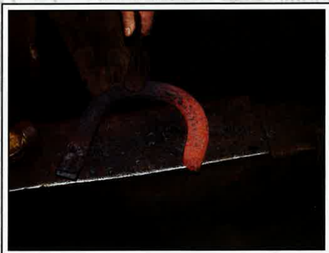
The quarter is formed while still on the second heat and is "boxed off" with the hammer on the outer margin from quarter to heel.
