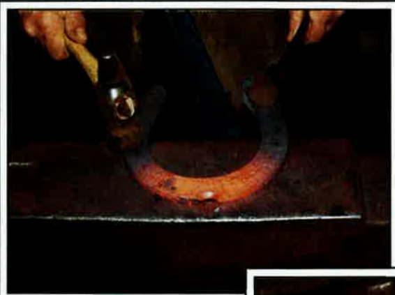
The nodule made with the clipping hammer is now ready to be drawn in a similar fashion to nodule created by the bob punch.
