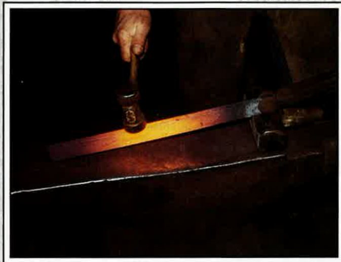
The initial toe bend being made with the essential long heat.
