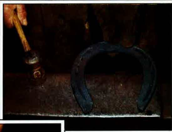
The finished article ready for fitting straight off the hammer and completed in four heats. Note the distinction between the inside web and the outside, the heel form and fullering. Spacing and pitch of the nail holes also differs considerably.
