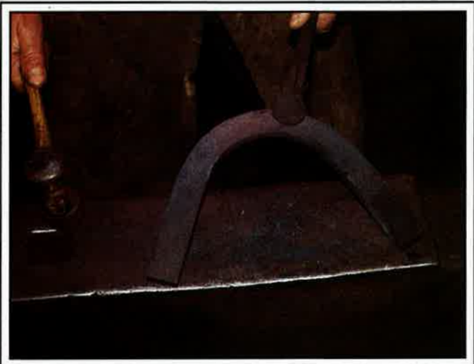
The completed toe bend. Everything flows from this and the shape should already conform with exact contour of the toe of the foot for which the shoe is intended. A good shoer must have the shape in the "mind's eye" right from the beginning.
