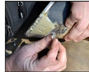
**Step 16:** Peel away the perforated sides of the Hanton blister, leaving the main portion of the blister covering the tab & glue. A rasp may be used to remove any small amounts of excess glue around the blisters.
