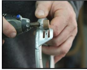
**Step 6:** For extra glue adherence, lightly grind or sand the outside of the tabs.
