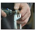
**Step 6:** For extra glue adherence, lightly grind or sand the outside of the tabs.
