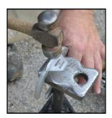
**Step 5:** Shape the Hanton Horseshoe to fit the hoof (as with any standard shoe), making sure the shoe is flat to the bottom of the hoof.
